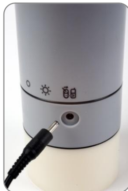
Fig. 9: Mobile phone charging socket
